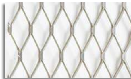
steel mesh embedded into the polyurethane core
